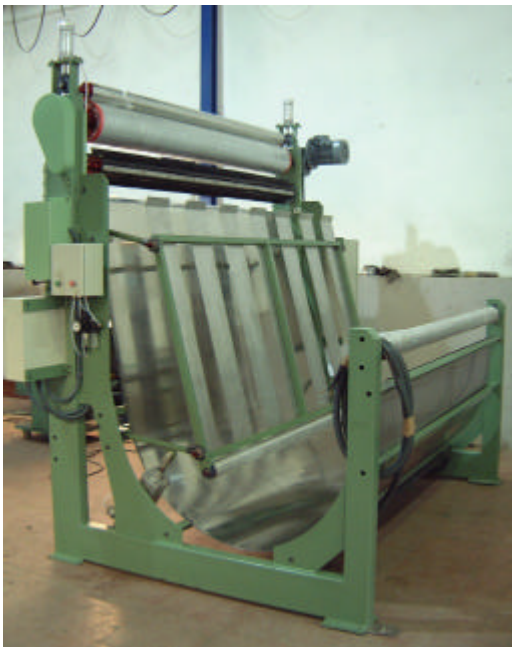
"J" type scray fabric accumulator with auto feeding compensator
