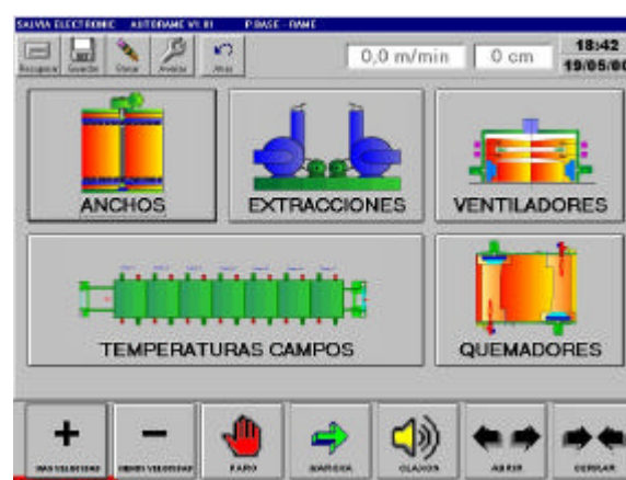
Drying chamber parameters control screen
